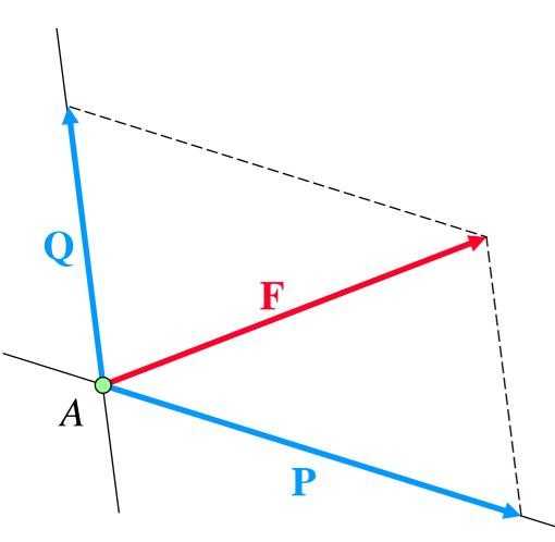
A force F can be resolved into two components P and Q by drawing a parallelogram which has F for its diagonal; the components **P** and **Q** are then represented by the two adjacent sides of the parallelogram and can be determined either graphically or by trigonometry.
