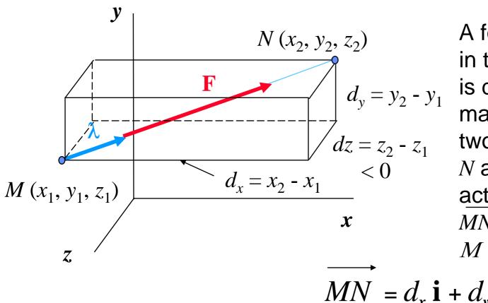
A force vector  $\mathbf{F}$ in three-dimensions is defined by its magnitude F and two points M and N along its line of action. The vector  $\overline{MN}$  joining points M and N is
