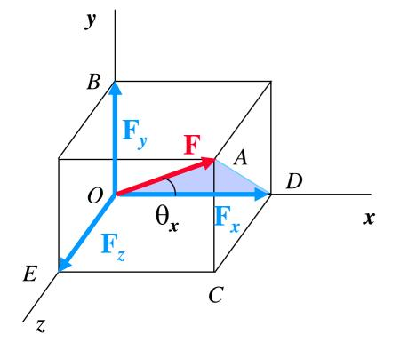
A force **F** in *three-dimensional space* can be resolved into components
