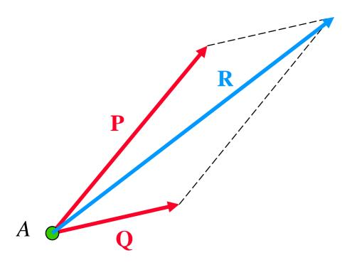
Any given force acting on a particle can be resolved into two or more *components*, i.e.., it can be replaced by two or more forces which have the same effect on the particle.
