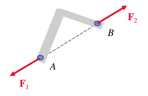
Two particular cases of rigid body equilibrium are given special attention. A *two-force body* is a rigid body subjected to forces at only two points. The resultants  $F_1$  and  $F_2$  of these two forces must have the *same magnitude, the same line of action, and opposite sense*.
