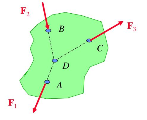
A *three-force body* is a rigid body subjected to forces at only three points, and the resultants  $F_1$ ,  $F_2$ , and  $F_3$  of these forces must be *either concurrent or parallel*. This property provides an alternative approach to the solution of problems involving a three-force body.
