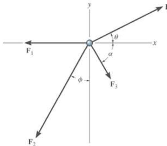
**Problem 2-2:** The gusset plate is subjected to the forces of four members. Determine the force in member  $B$  and its proper orientation  $\theta$  for equilibrium. The forces are concurrent at point  $O$ .
