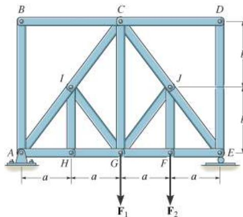
**Problem 5-6:** Determine the force in members  $CD$  and  $GF$  of the truss and state if the members are in tension or compression. Also indicate all zero-force members.
