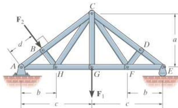
**Problem 5-7:** Determine the horizontal and vertical components of force that pins A and C exert on the frame.
