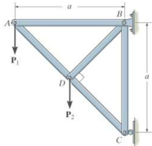
**Problem 5-2:** Determine the force in each member of the truss and state if the members are in tension or compression.
