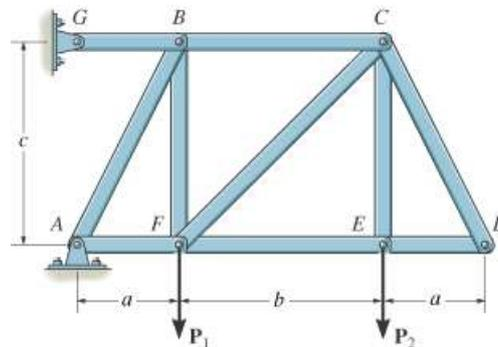
**Problem 5-3:** Determine the force in each member of the truss and state if the members are in tension or compression.
