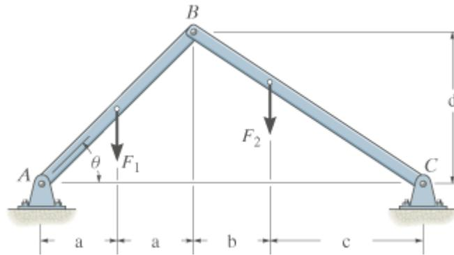
**Problem 5-8:** Determine the horizontal and vertical components of force which the pins at A, B, and C exert on member ABC of the frame.
