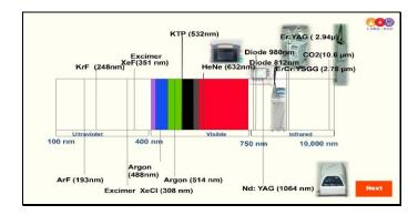
Slide 9 - laser wavelength and laser machine
