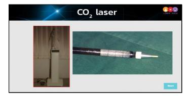
Slide 12 - CO2 laser hollow wave guide
