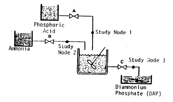
The continuous process has shown in the Figure above. In this process, the phosphoric acid and ammonia are mixed, and a non-hazardous product, diammonium phosphate (DAP), results if the reaction of ammonia is complete. If too little phosphoric acid is added, the reaction is incomplete, and ammonia is produced. Too little ammonia available to the reactor results in a safe but undesirable product.
