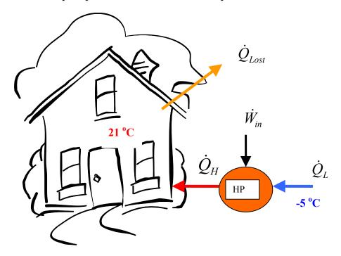
The heat lost by the building has to be supplied by the heat pump.
