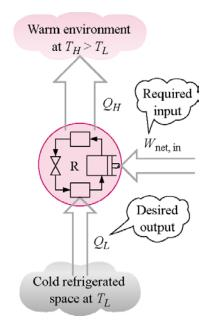
For the refrigerator the desired result is the heat supplied at the low temperature and the input is the net work into the device to make the cycle operate.
