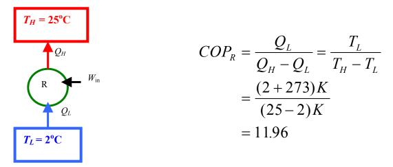
The claim is false since no refrigerator may have a COP larger than the COP for the reversed Carnot device.
