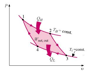
You may have observed that power cycles operate in the clockwise direction when plotted on a process diagram. The Carnot cycle may be
