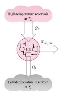
The thermal efficiency of the above device becomes
