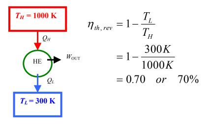
The claim is false since no heat engine may be more efficient than a Carnot engine operating between the heat reservoirs.
