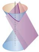
Parabola: plane parallel to side of cone
