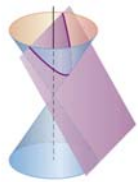
Parabola: plane parallel to side of cone
