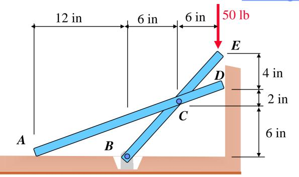
For the frame shown and neglecting the effect of friction at the horizontal and vertical surfaces, determine the forces exerted at *B* and *C* on member *BCE*.
