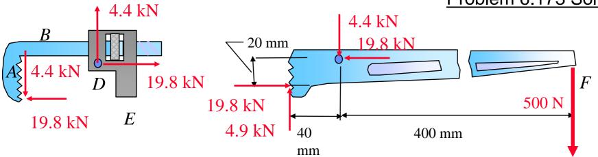
All components act in the directions shown. Components on the pipe are equal and opposite to those on the wrench.
