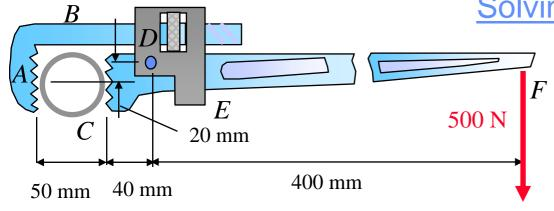
A pipe of diameter 50 mm is gripped by the Stillson wrench shown. Portions *AB* and *DE* of the wrench are rigidly
