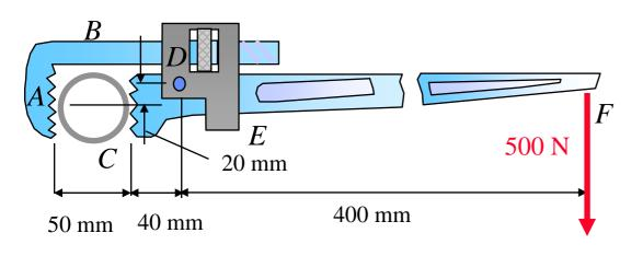
A pipe of diameter 50 mm is gripped by the Stillson wrench shown. Portions *AB* and *DE* of the wrench are rigidly
