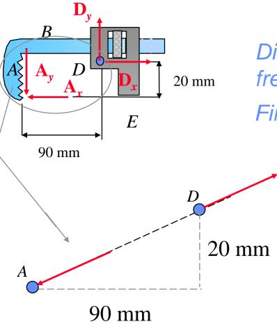
Dismember the machine, and draw a free-body diagram of each member.
