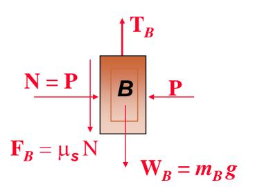
Since motion is impending,  $F = F_{\rm m} = \mu_{\rm s} N$ . Substituting for  $\mu_{\rm s}$  its known value, you can express F in terms of N on the free-body diagram, thus eliminating one unknown.
