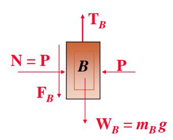
Assume a possible motion of the body and, on the free-body diagram, draw the friction force in a direction opposite to that of the assumed motion.
