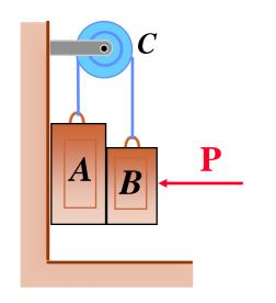
Block *A* of mass 12 kg and block *B* of mass 6 kg are connected by a cable that passes over pulley *C* which can rotate freely. Knowing that the coefficient of static friction at all surfaces of contact is 0.12, determine the smallest value of *P* for which equilibrium is maintained.
