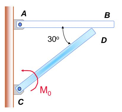
Two uniform rods each of weight W and length L are maintained in the position shown by a couple  $\mathbf{M}_0$  applied to rod CD. Knowing that the coefficient of static friction between the rods is 0.40, determine the range of values of  $\mathbf{M}_0$  for which equilibrium is maintained.
