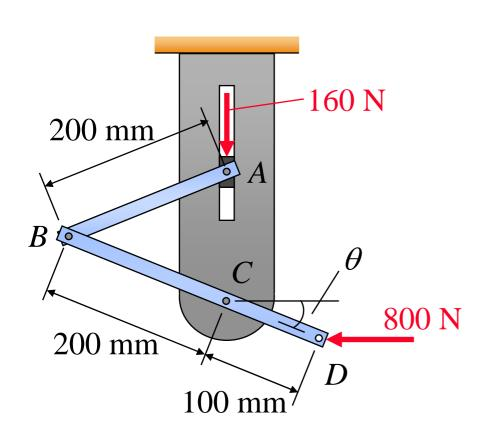
Rod AB is attached to a block at A that can slide freely in the vertical slot shown. Neglecting the effect of friction and the weights of the rods, determine the value of  $\theta$  corresponding to equilibrium.
