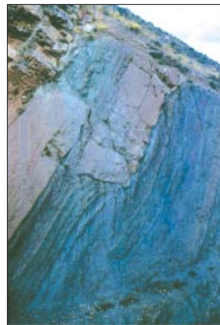
Anisotropic heterogeneous rock mass – Mequinenza region, Spain
