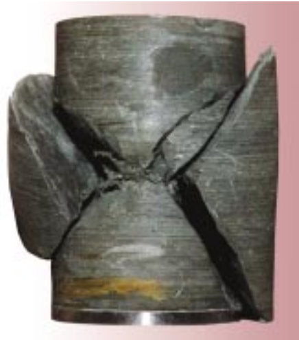
Photo 3 - Specimen after failure in triaxial test (French standard p 94-422)
