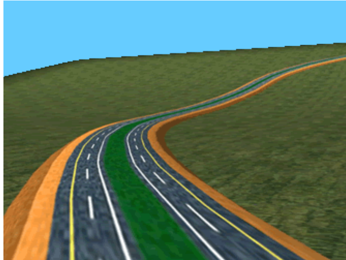
A: Broken-back curve
