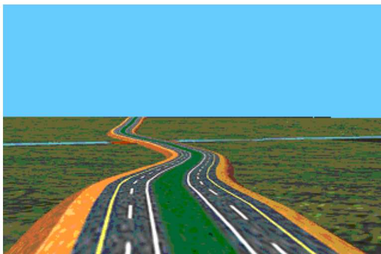
A: Distorted alignment to create square river crossing
