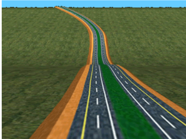
A: Short hump and dip preceding horizontal curve
