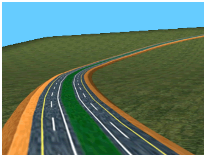
B: Replacement of broken-back curve by single radius long curve
