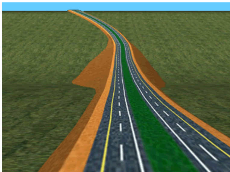
B: Long sag curve linking into horizontal curve
