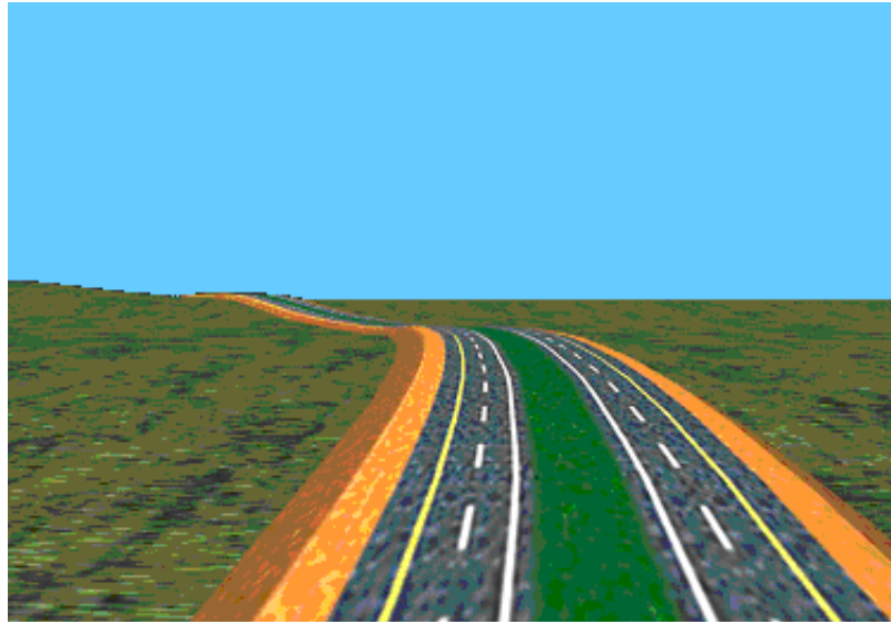
A: Short humps on long horizontal curve
