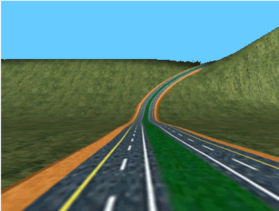
Figure 5-10: Out-of-phase vertical and horizontal alignments
